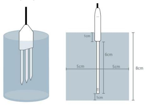
As shown in the figure, the height of the cylinder is 8cm, the radius is 5cm, and the length of the probe is 1cm deep in the water. Avoid big rocks or tree roots within this effective range.
